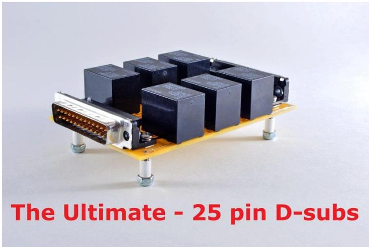
The D-sub connectors' pins are rated at 5 amps continuous. The Omron relays are rated at 10 amps continuous. The flap relay traces have been designed to conduct 5 amps continuously in keeping with the draw of the Usher Enterprises (Van's Aircraft) flap motors or our own RV Flap Actuators. CAUTION: It is important to use the designated pin-outs for the flaps, pins 6 and 8, in the 25-pin connectors as shown in the attached schematic, as this circuit is designated to handle the flap motor
