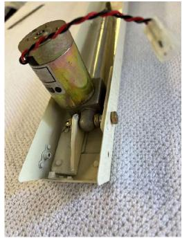
**Remove the Motor –** Remove the ½" bolt, castle nut, and cotter key.
