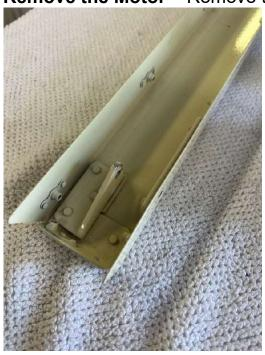
**Drill Out Old Brackets –** Remove the old bracket, shim, and doubler on the side of the channel. Remove the two nutplates shown on the sides of the flap channel. You will reuse the attach angle shown clecoed below. You can also reuse the nutplates but now they will be attached to new brackets (see below).
