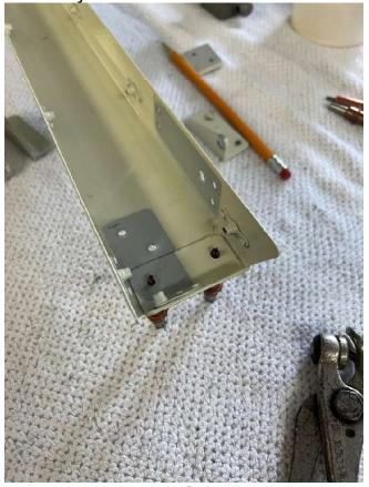
**Reinstall the Flap Channel –** temporarily mount the flap channel in the airplane (RV-7 in this example). Position the new brackets as shown below leaving about 1/8" spacing around the brackets as shown in the photos.
